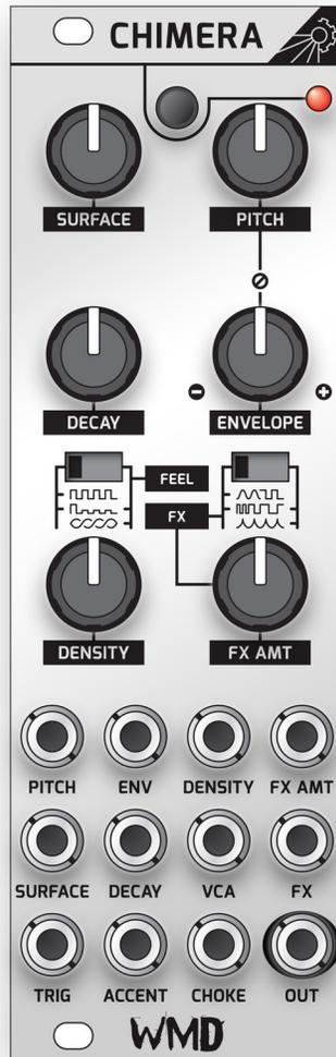
**PITCH:** Shift the frequency of the metal texture here. The pitch control spans 5 octaves, and every pitch setting produces its own range of usable metal timbres.
